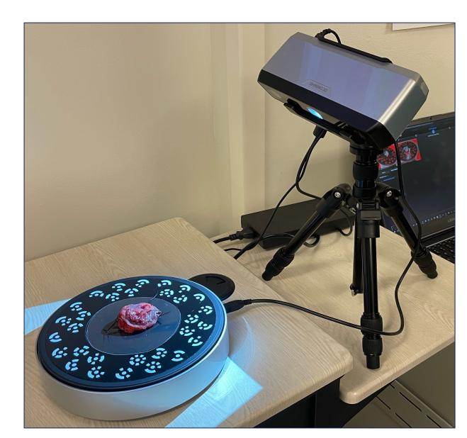
Figure 2b. Intraoperative EinScan 3D Scanner Setup (Different Specimen Pictured than in Figure 2a)
