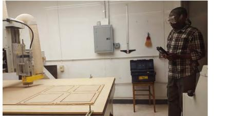
Figure 18: CNC Panel Frame and Construction
