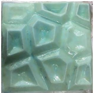
Figure 33: Fiberglass Composite Mold
