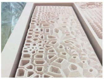
Figure 30: CNC'd Model Foam Facade Representation
