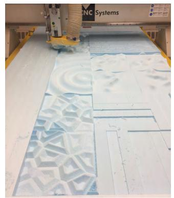
Figure 31: CNC Milling the Mold
