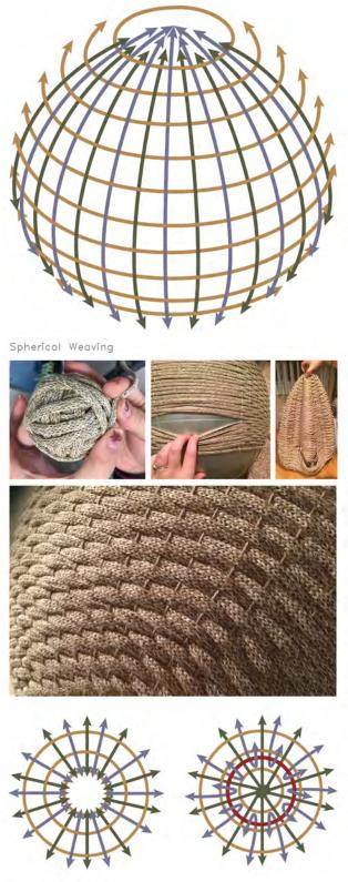
Connection Points Figure 11: Weaving Pattern Of The Interior Sleeping Pod
