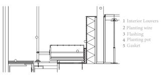
Figure 13: Wall assembly detail
