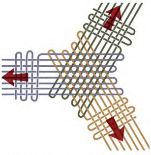
Traditional Weave on all sides to create the straps Figure 13: Hexagonal Woven Straps
