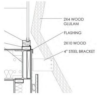
Figure 20: Louver Connection Detail
