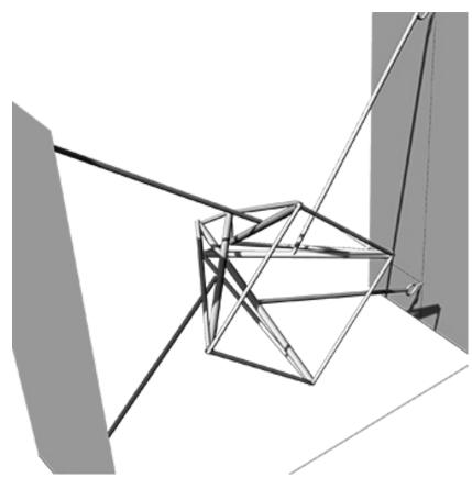
Figure 4: Digital Model showing tensegrity module at rested state
