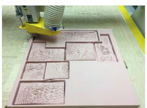
Figure 27: CNC Milling the Facade Iterations
