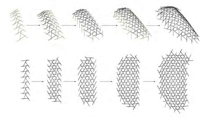
Figure 12: Assembly method of reciprocal structure
