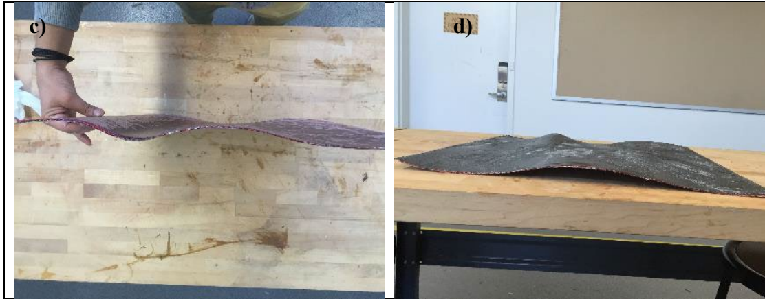
Figure 6.1 Curved Panel formation on Static Mold a) Wooden board CNC milled mold b) Hand lay-up of composite materials and matrix c) Final free form double curved panel d) Final free form double curved surface (Pictures courtesy Gurjar)
